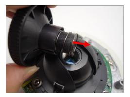
4. Remove the transparent plastic from the replacement lens.
