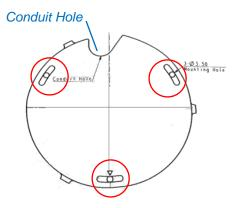
**NOTE:** Depending on the surface where you will install the camera, it may be necessary to drill three (3) holes with  $\phi$  3.5 on the ceiling and use the supplied screw torx.
