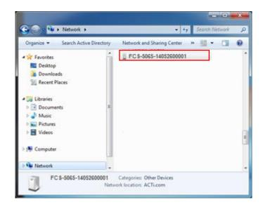
By double-clicking with the left mouse on the camera model, it is possible to automatically launch the default browser of the PC with the IP address of the target camera filled in the address bar of the browser already.
