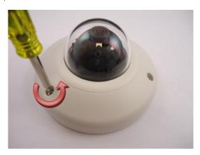
2. Push the clips outwards to release the dome cover latches.
