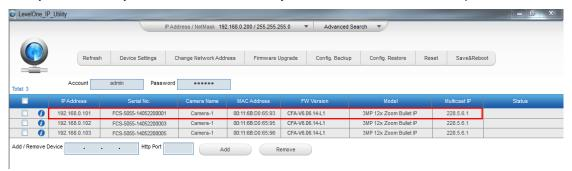
You can quickly see the camera model in the list. Click on the IP address to automatically launch the default browser of the PC with the IP address of the target camera filled in the address bar of the browser already.
