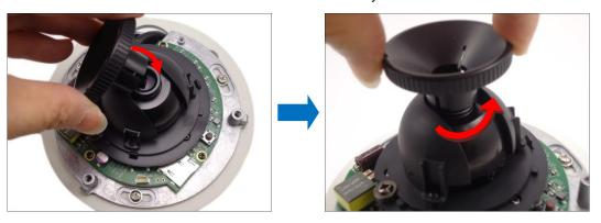
3. When the lens comes off, remove the spring and remove the bundled lens from the lens focus tuner.
