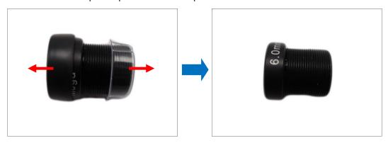
5. Attach the spring to the replacement lens.
