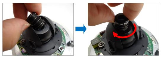
7. Attach the lens focus tuner when the tip of the lens is difficult to hold then turn it clockwise or counter-clockwise to adjust the camera focus. See *How to Adjust the Viewing Angle and Focus* on page 15 for more information.
