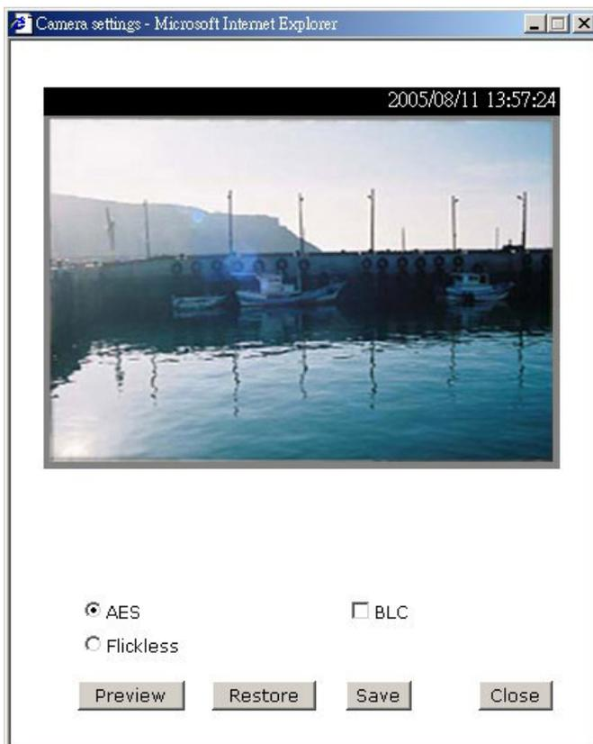
**"AES"** - auto electronic shutter, enable this will let CCD sensor adjust electronic shutter automatically. Disable this when auto iris lens is attached.
