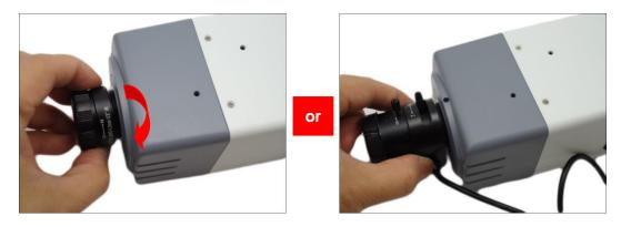
4. For cameras models FCS-1152, connect the lens cable to the DC-iris port.
