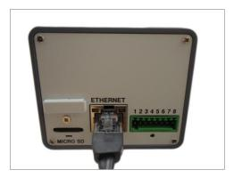
If necessary, connect audio input/output or DI/DO devices to the camera. See How to Connect DI/DO and Audio Devices (Optional) on page 10 for more information.
