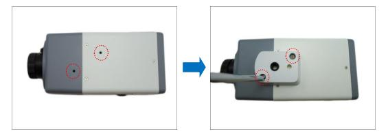
• If the camera will be installed on the wall, attach the mounting block on the bottom side of the camera. Secure the mounting block to the camera using the two (2) screws included in the mounting block package.
