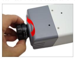
2. Twist and pull to remove the cap from the threaded end of the replacement lens.
