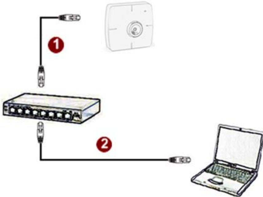
**Please use a PoE (Power over Ethernet) supported switch or injector:**
