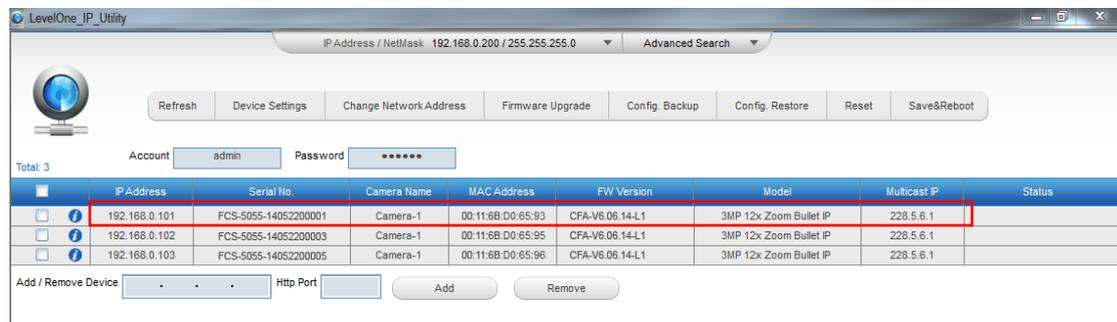
You can quickly see the camera model in the list. Click on the IP address to automatically launch the default browser of the PC with the IP address of the target camera filled in the address bar of the browser already.
