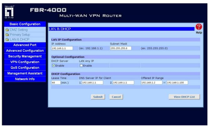
Figure 2-3: LAN & DHCP Setup
