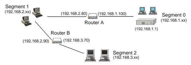
Figure 4-3: Routing Example
