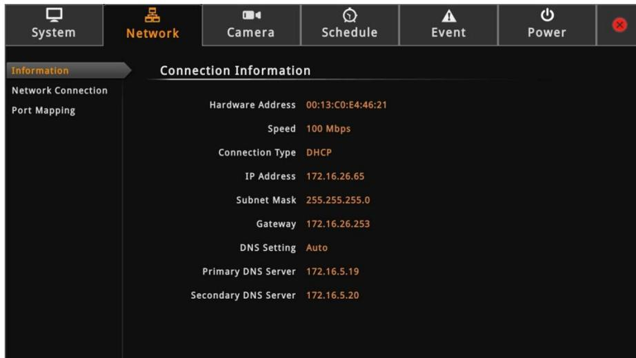
The network information, such as the **Hardware Address** (MAC address), **Speed**, **Connection Type**, **IP Address**, **Subnet Mask**, **Gateway**, **DNS Setting**, and **Primary** and **Secondary DNS Server** are displayed.
