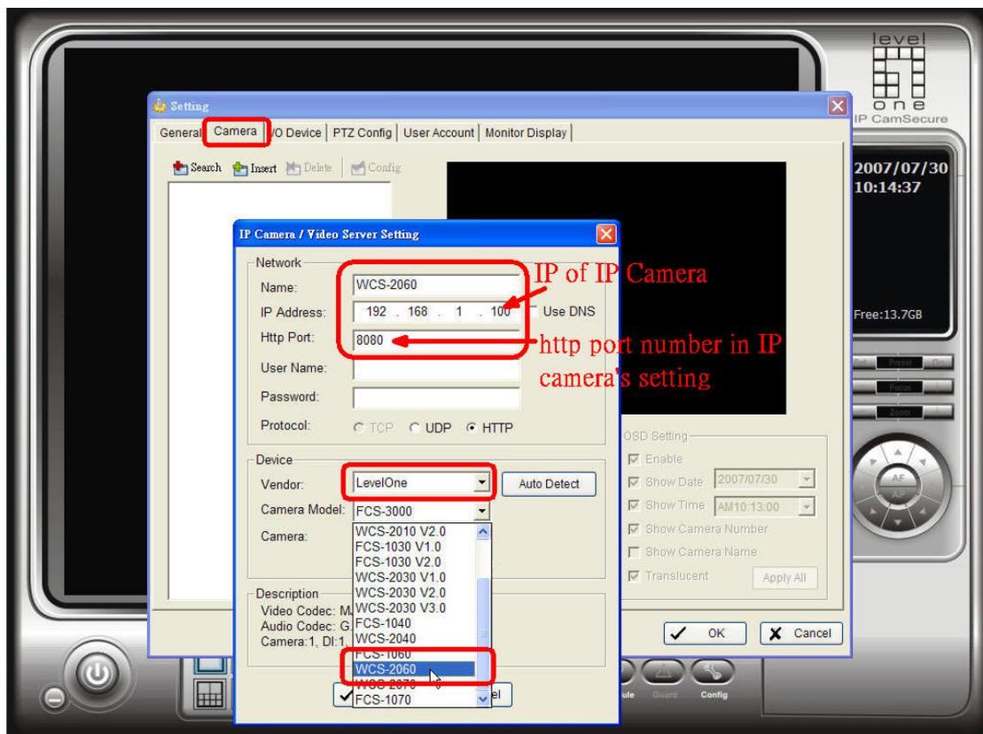
Type in the name, IP of IP Camera, the defined Http Port number, the User and Password account on IP Camera. Go to Device section and select the respective Camera Model. Note: you have to match the settings in your IP camera with the settings here.
