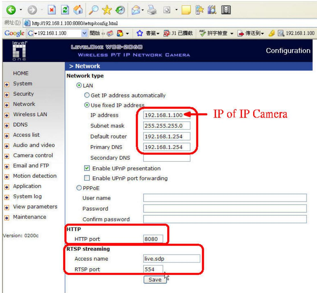
In the picture above, the network setting of WCS-2060 is displayed. In order to make IP CamSecure software work, user has to be consistent in the parameter settings of IP CamSecure and those in IP camera device.
